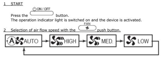
Pressing the button changes the operating modes in the order shown in the picture. When the air speed is set to "AUTO", the fan speed varies depending on the room temperature. By default, this function is set on the central control unit. We recommend using this feature.
