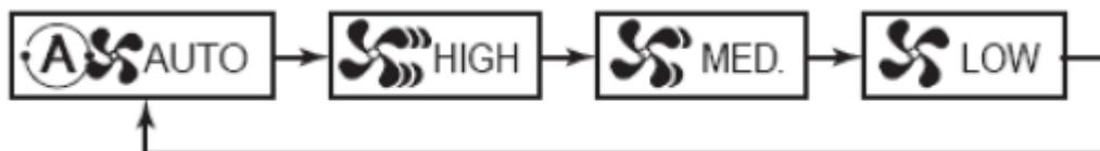
Pressing the button changes the operating modes in the order shown in the picture. When the air speed is set to "AUTO", the fan speed varies depending on the room temperature. By default, this function is set on the central control unit. We recommend using this feature.
